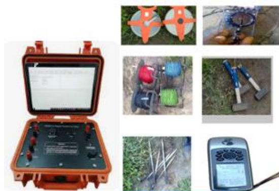
Figure 6: Resistivity meter and other field equipment used.
